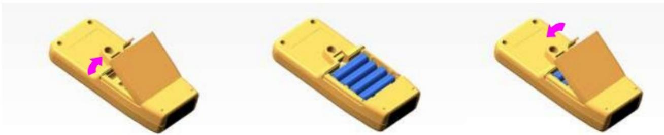
Lift the cover while pushing down the clip.
