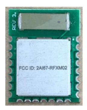
TMWRFX-M-CHIP is a wireless module. Designed based on the TI CC1310 high-performance wireless transceiver chip, is a two-way wireless receiving and transmitting module. The Wireless frequency is 433.92MHz
