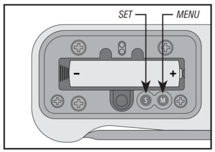
To change any of these settings, loosen the battery cover screw using a Phillips screwdriver and remove the battery cover. Open the probe to turn the unit on. Thermapen ONE has two small buttons inside the battery
