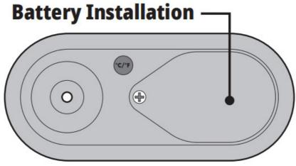
Replace the battery when low battery symbol 'Bat' flashes.
