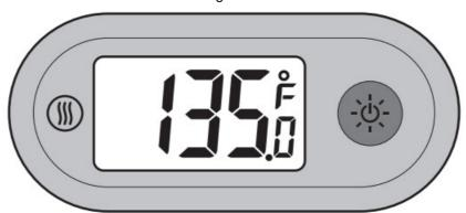
Insert the stainless steel probe to the desired depth. The measured temperature will be shown on the LCD display within 2-3 seconds.
