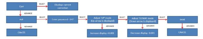
Selecting Add will display a password field of 3 digits. Enter the password (247) one digit at a time using the ADVANCE button to increment each display digit. Then use the SELECT button to go to the next digit. Pressing SELECT for the 3" digit will take you to a temperature display where you can adjust the displayed temperature. The arrow indicator shows the direction you are changing the temperature. Press and hold the ADVANCE button to
