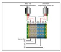
In order to avoid EMI issues with a temperature controller, the shield of the control wire shall be connected to the instrumentation earth only. Do not connect the control wire shield in the junction box.
