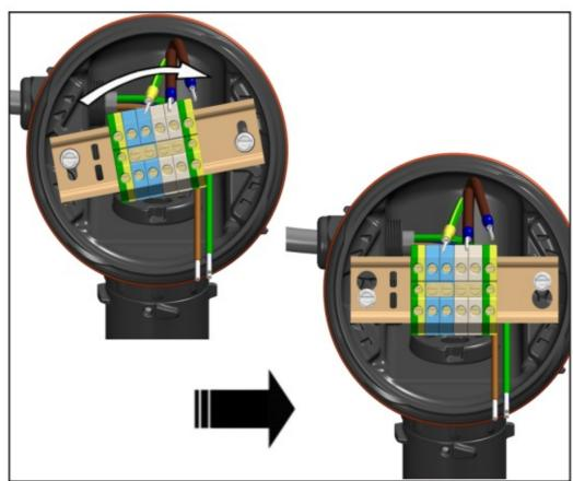
14. Install junction box lid and twist hand tight. Insert screwdriver into ratchet slots located on side of junction box base.
