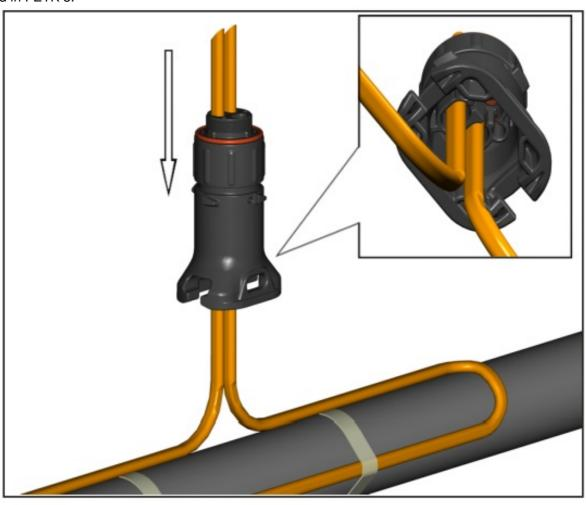
For HPT and FP cable, exchange grommet in Terminator with GRW-G provided in PETK-3.
