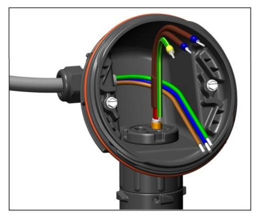
13. Install terminal block and complete system wiring. Terminal set screws shall be tightened to a torque value of 1.4 Nm (12.4 lb-in). See below for wiring details.
