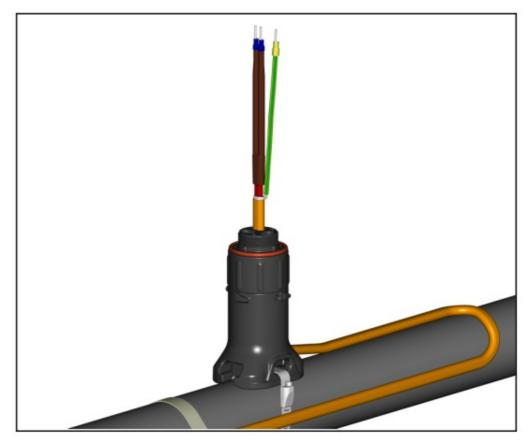
9. Push excess cable back through expediter. Tighten cap securely. Tape cable expansion loop to pipe.
