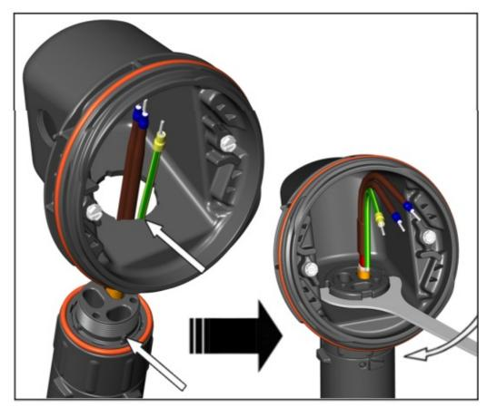
11. Remove M25 dust cap. Install M25 power gland (order separately) and M25 blind plug. For in-line splice, T-splice, or end termination, install additional M25 blind lug (order M25-B-EXE separately) instead of M25 power gland.
