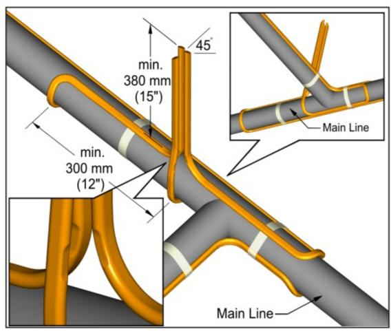
Insert three cables into expediter. Note: For HPT and FP cable, exchange grommet in Terminator with GRW-G provided in PETK-3.
