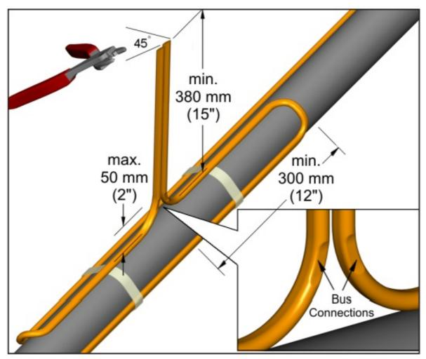
Insert two cables into expediter. Note: For HPT and FP cable, exchange grommet in Terminator with GRW-G provided in PETK-3.
