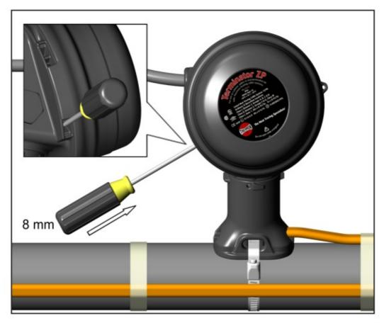
15. Use screwdriver to ratchet on junction box lid. Lid will rotate 30 degrees.
