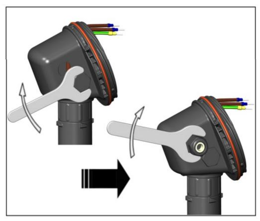
12. Install power cable (if necessary).
