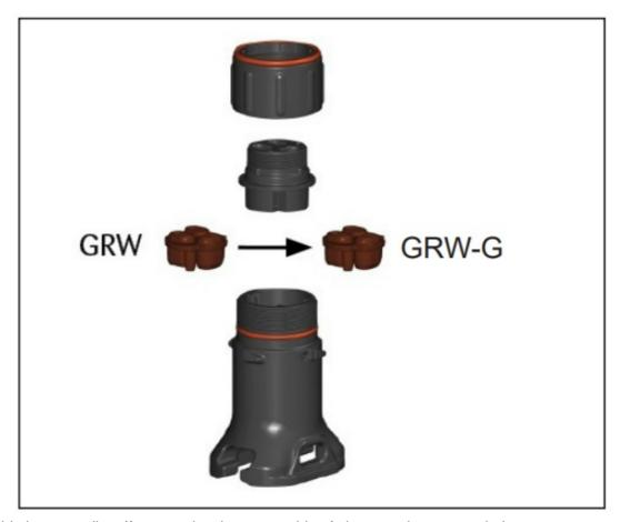
3. Insert cable into expediter. If mounted on bottom or side of pipe, punch out weep hole.
