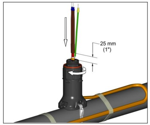
10. Mount junction box base on expediter. Make sure to align slots to properly orient junction box base. Tighten nut with Terminator-LN-Tool. If mounting horizontally, threaded gland holes must face downward.
