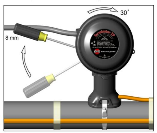
16. Lid latch mechanism fully engaged. To remove lid, repeat steps 14 and 15 but in the opposite direction.
