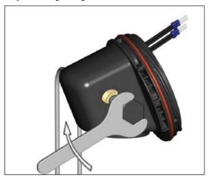
8. Install M25 power gland (customer supplied) in M25 threaded entry. For in-line splice or 3-phase wye connection, install M25 blind plug (order M25-B-EXE separately) instead of M25 power gland.
