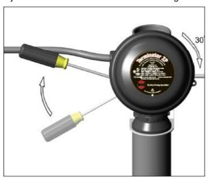
15. The lid latch mechanism is fully engaged. To remove the lid, repeat steps 12 and 13 but in the opposite direction.
