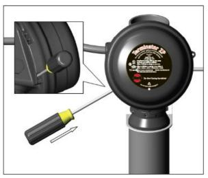
14. Use a screwdriver to ratchet the junction box lid. The lid will rotate 30 degrees.
