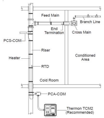
In case of dry type, the tracing is meant to keep the empty branch pipes above freezing point, so that when upstream control valve operates the pipe body does not cool down the incoming water.
