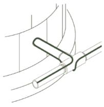
4. All of the heat trace power connection points should be secured to the piping. Heat trace should not pass through the air to travel to an adjoining pipe. Instead, use multiple circuit fabrication kits interconnected with conduit and field wiring as shown.
