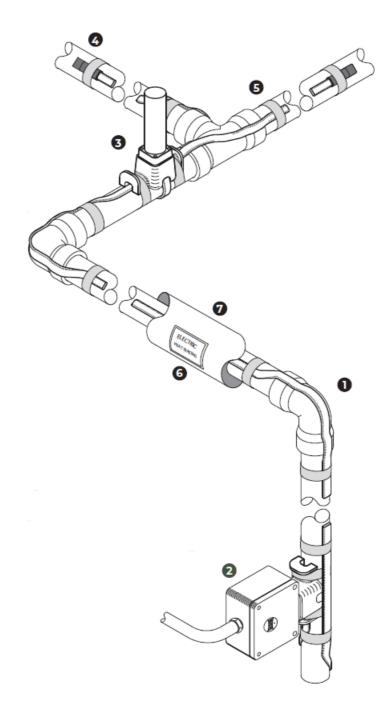
An FLX self-regulating freeze protection heat tracing system will typically include the following components:
