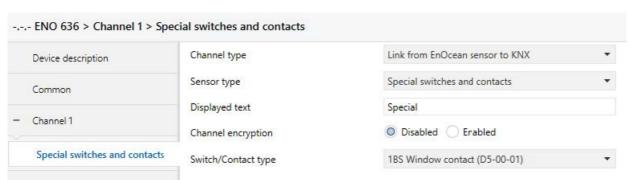
For window contacts, up to 4 contacts can be taught into one channel. The gateway detects a common state of all contacts learned in the channel and sends the value "closed" only when all windows are closed.
