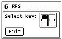
When emulating an RPS switch, the learning mode in the gateway is activated by pressing T2 long at the desired channel. The "Select key:" selection appears in the display. The pressure point (top or bottom) of the learning telegram can be selected here with the T2 button. For some actuators, several pressure points must be separated separately.
