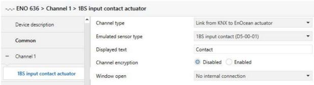
With this profile, a 1BS contact input is emulated, this profile is e.g. used by many simple EnOcean window contacts. One object is available:
