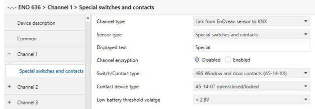
For this device type, up to 4 contacts can be taught into one channel. The gateway detects a common state of all contacts learned in the channel and sends the value "closed" only when all windows are closed. The following devices of this profile family are supported:
