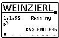
The repeater function of the STC-KNX is activated by the general parameters in the ETS. If the function is enabled it will be displayed in the main menu of the display left under the individual address.
