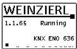
The integrated display is used for commissioning and system diagnostics. In normal operation, it is not required and is not visible when the device is closed.
