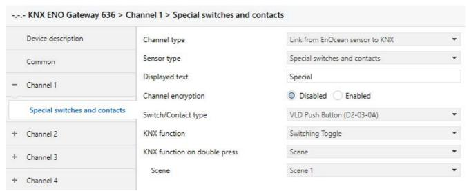
This profile supports push buttons with short/long and double key press. The following object is available for monitoring the battery status:
