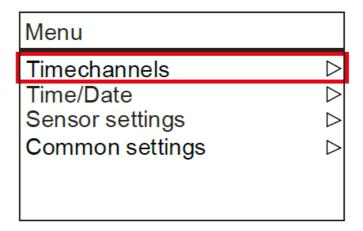
Up to 3 time channels with 4 time periods each can be parameterized. The time channels are prioritized, channel 3 has the highest priority.
