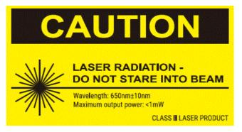
• The maximum output power emitted through the laser aperture is 85uW.
