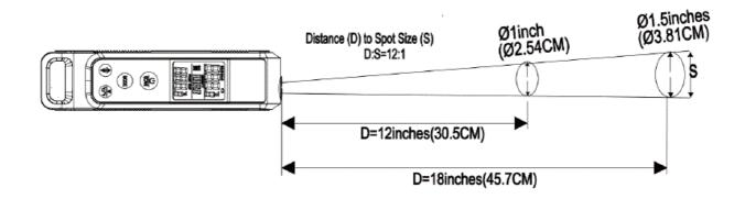
For the most accurate results, make sure the target has a surface area of twice the corresponding spot diameter. Insufficient surface area will result in inaccuracies. For example, if you use a device with DS ratio 12 to measure an area with a diameter 1 inch (or 25.4mm), the recommended distance to hold the thermometer from the surface of
