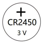
Battery positive pole This side outside when installing the battery
