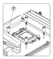
Install four 115X standoffs through backplate screws from front side of motherboard
