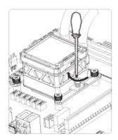
Secure waterblock on CPU with two nuts on waterblock bracket
