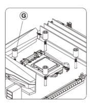
Install four 1700 standoffs through backplate screws from front side of motherboard
