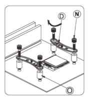
Secure two AM4/AM5 brackets with four AM4/AM5 screws.
