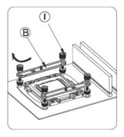
Install two Intel brackets on LGA20XX screws, secure them with nuts.
