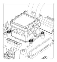
Secure waterblock on CPU with two nuts on waterblock bracket
