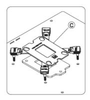
Install Intel backplate backplate from back side of motherboard
