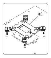
Install adjusted intel backplate from back side of motherboard
