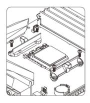
Remove factory CPU brackets and screws, KEEP the backplate
