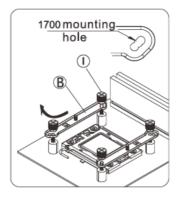
Install two Intel brackets on standoffs, secure brackets with four nuts.
