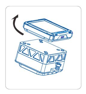
Magnetic Waterblock Panel can be adjusted to four directions.
