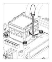
Secure waterblock on CPU with two nuts on waterblock bracket
