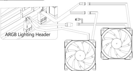
For Fans with ARGB lighting, to control the ARGB lighting, connect the ARGB lighting cable (3-pin +5V) to the motherboard ARGB lighting header or ARGB lighting controller, lighting effects can be synced by connecting fan lighting headers with each other.
