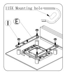
Apply thermal paste on CPU, install the heatsink with a screw driver, and install fans on heatsink with fan clips, Place LCD panel on top of heatsink.
