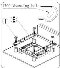
Apply thermal paste on CPU, install the heatsink with a screw driver, and install fans on heatsink with fan clips, Place LCD panel on top of heatsink.
