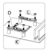
Remove AMD plastic brackets, KEEP the backplate, install AM4/AM5 metal brackets on AM4/AM5 spacers with AM4/AM5 screws.
