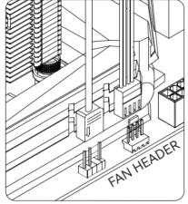
Connect 4 pin PWM fan cable to motherboard CPU\_FAN header, use Fan Y-Cable to sync fan speed for dual fan setup.
