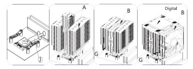
Apply thermal paste on CPU, install the heatsink with a screw driver, and install fans on heatsink with fan clips, Place LCD panel on top of heatsink.
