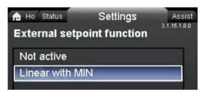
Figure 18: Press "Ok" to select Linear with MIN
