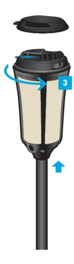
**3. Turn on:** Rotate torch collar to the right until indicator line points to flow. The gas will start to flow. Wait 5 to 10 seconds then rotate torch collar until indicator line points to "START" and you hear a clicking sound. To verify that the torch has been activated, look in the oval view hole located on the torch collar to the right of the "START" button.
