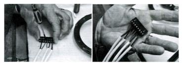
Warning: Be sure connectors are plugged in correctly, do not shift over one pin.
