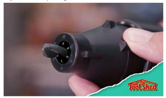
2. Hold back the toggle and position the sleeve into the depth adjustment cylinder. Push the drill bit in as far as it will go.
