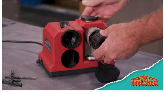
6. Rotate the sleeve back and forth until there is minimal contact with the grinding wheel.
