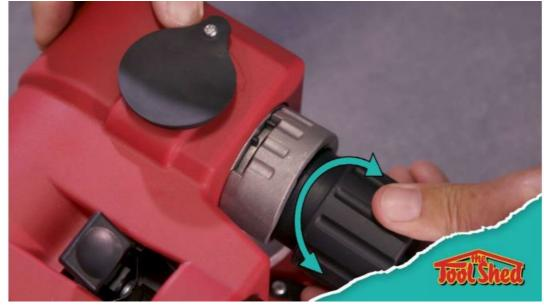
7. Remove the sleeve from the cylinder, rotate it 180°, put it back into the cylinder, and repeat the process.
