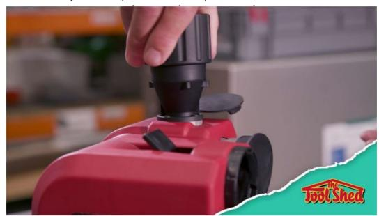
3. Rotate until minimum contact, take out and rotate 180°, place back in and repeat the process.
