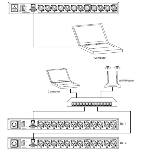
• The illustrations show schematically how one device or several devices can be integrated into a local area network (LAN).
