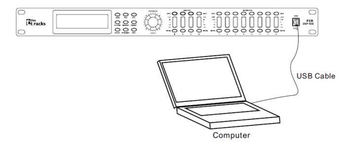
• The figure schematically shows how the device can be controlled via a computer's USB port.
