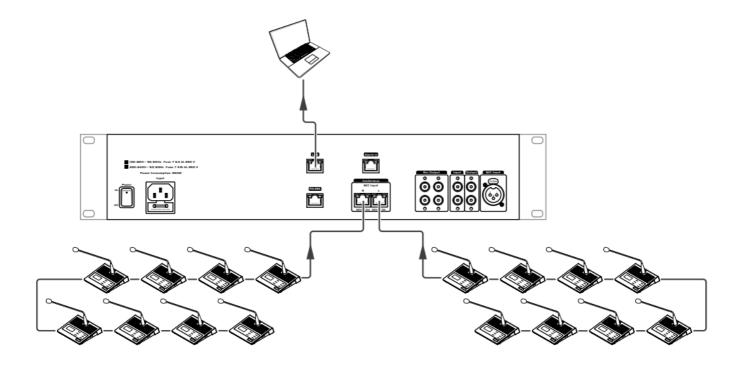
Up to 16 call stations can be connected in 2 lines to the control centre
