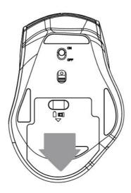
• Open the battery compartment, remove the paper tab and USB receiver. Insert the batteries following the
