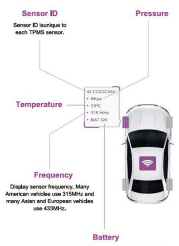
Sensor battery status is displayed. If a sensor's battery is suffcient "OK" will be displayed. If a sensor battery is low, "NOK" will be displayed.
