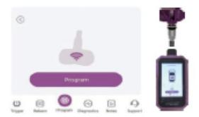
• Place the sensor above the tool's antenna, and tap program.
