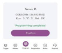
Once successfully programmed, the tool will display the sensor's ID, pressure, temperature and battery status.
