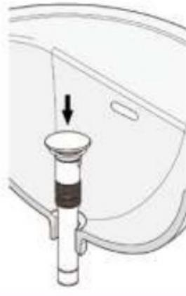
3. Screw components A & B back on as shown.
