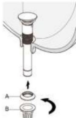
4. Connect the rear end of the drain to the Drain Pipe.
