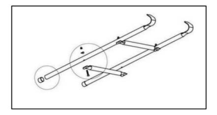
Layout all of the parts as pictures. select two frame pole which have two or three holes.
