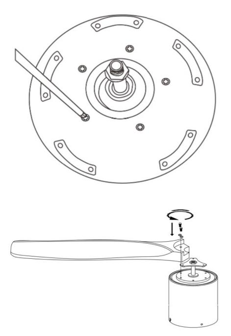
Before installing fan blades, remove the motor's fastener that is only used to protect the motor from damages in transit then install fan blades on fan's motor, align holes of blades and motor, then screw blades with provided screws.
