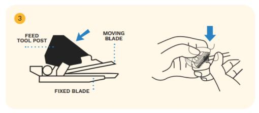
3. The white moving blade can be clicked down, and then you can clean the hair between the moving blade and the fixed blade.
