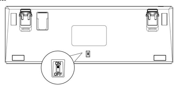
Switch to ON, In 2.4G mode, holding down seconds, and then search for "2.4G Wireless Device" in the device systems to connect the keyboard.
