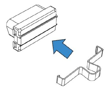
Do not use screwdrivers or other tools to lever and disconnect the device.
