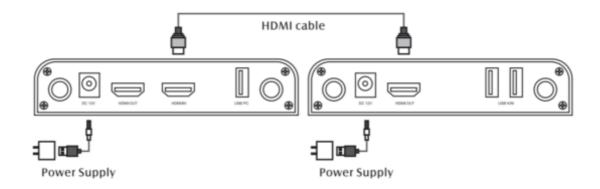
Step 1: Plug In the power adapters of both TX & RX
