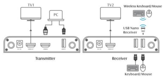
Step 1: Connect PC to TX with USB & HDMI cables
