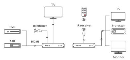
Step 1: Connect the IR receiver to the RX
