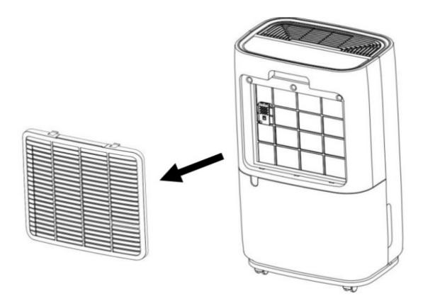
• Rinse under a running water or using the vacuum to clean the dust
