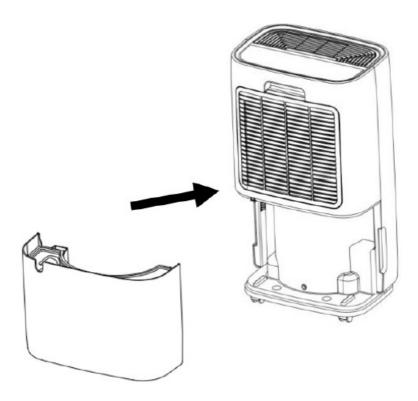
• Do not discard the magnets and plastic rivets in the tank. Otherwise, the dehumidifier cannot be started, or the machine will not automatically stop working when the water tank is full, and the condensed water overflow will damage the floor of the room.
