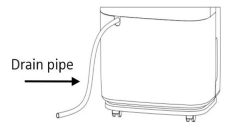
Please do not block the drain or drain pipe, if blocking phenomenon, condensed water will flow into the tank. Please do not bend the drain pipe. The height of the drain pipe should be lower than the outlet. The drain pipe must be firmly connected to the outlet.
