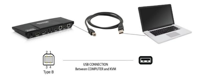
Once the connection is established you should have the "Online Light" on this indicates the connection is active this is what makes the communication between the peripherals(Mouse, keyboard, USB devices) and the computers.
