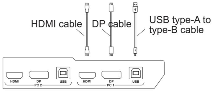
**Note:** Both Input A and input B should be connected to the same computer. If connect only one of them, then the dual monitor function would not work properly.
