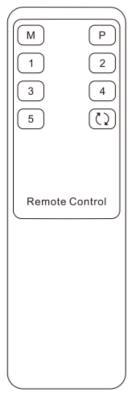
M: Switch images on the Display B P: Switch images on the Display A
