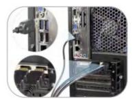
2. Connect external mouse and keyboard to KVM's keyboard and mouse input port.
