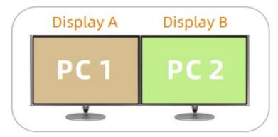
**Tips:** When different PCs are displayed on different monitors, you can double-click the Right-[Alt] on the keyboard connected to the KVM to switch the focus between different PCs.
