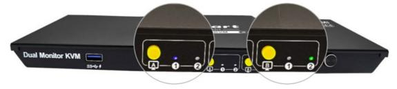
• Press [A]/[B] button to switch between PCs on corresponding monitor on display mode 2.
