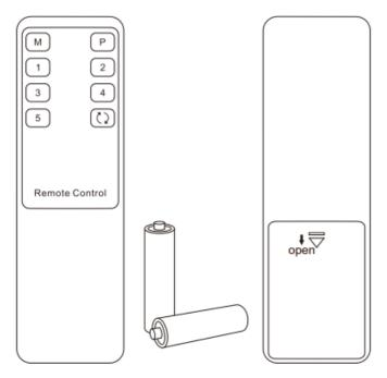
**Tips:** By default, the remote control is not equipped with batteries, due to the safety requirements of some express companies. Install AAA dry cells before use.
