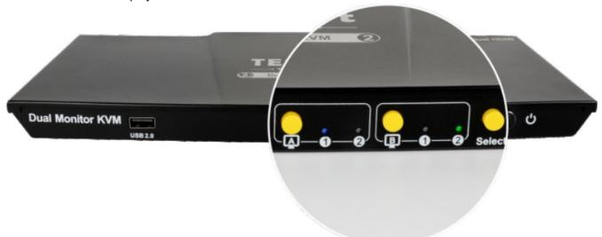
The 2×2 Dual Monitor KVM Matrix Switch has two different colored lights to indicate the status of the different input sources.
