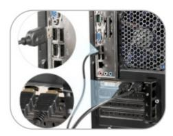
2. Connect external mouse and keyboard to KVM's keyboard and mouse input port.
