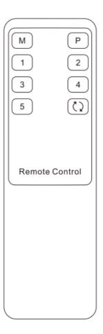
M-Turn on/off the Smart EDID Management in Display Mode 2 P -Switch the keyboard and mouse focus between PC1 and PC2 in Display Mode 2
