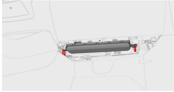
3. Disconnect the electrical connector from the front passenger knee airbag.
