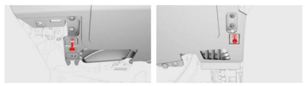
2. While supporting the front passenger knee airbag, remove and discard the bolts (x4) that attach the front passenger knee airbag to the instrument panel.
