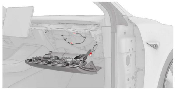
3. Remove the glove box from the vehicle.
