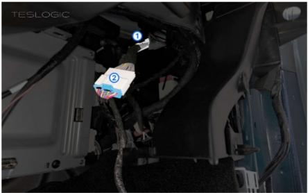
3. Connect the upper and lower wiring harnesses by attaching the corresponding plugs.
