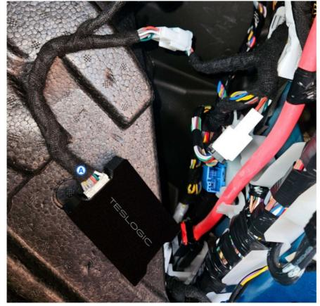
5. Place Teslogic Pro device in the recess below.
