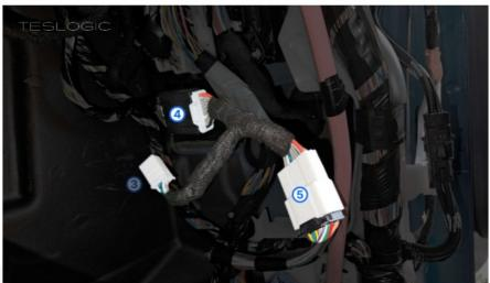
2. Disconnect the plug from the upper connector, connect it to the long wiring harness and then connect the long wiring harness to the upper connecto
