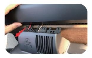
For Right-hand drive vehicles: need to install adhesive tape (two to three layers) to adjust the screen position until it appears to be at a basic horizontal level with the original vehicle screen when viewed from the right side. (Please note that a slight tilt may occur during the installation for right-hand drive vehicle, which is normal)
