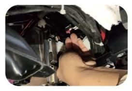
• Insert the connected plug into the original position of the OBD plug
