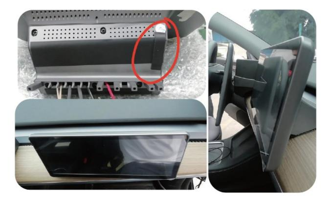
• The base here must be pressed to the bottom, make sure to insert the buckles in parallel when installing, if not
