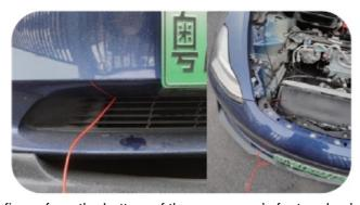
3. Find the rubber circle in the figure from the bottom of the passenger's foot and poke a small hole in the rubber, Thus, put the plug out of the front cover from here, and connect the plug with the plug connected with the "front camera" plug of our display in the car, and the installation can be completed.
