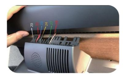
• The wiring harness installation effect is shown in the figure. If any wiring harness is installed incorrectly, it will cause the risk of wiring harness damage (the number marked on each wiring harness is the position of the corresponding hole).
