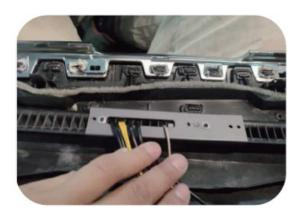
• After fixing the plate, insert the plugs corresponding to all colours,
