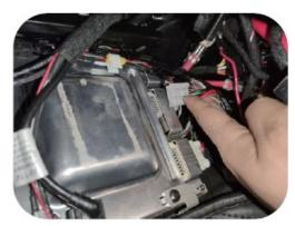
• Connect the OBD plug to the female plug of the Y-type plug provided by us
