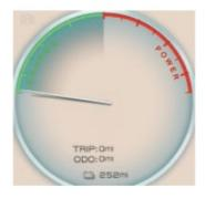
The single mileage, total mileage and remaining mileage information are displayed under the power instrument.
