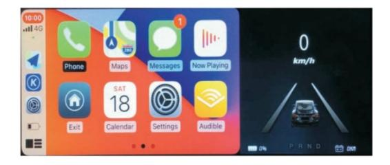
The screen projection interface can be displayed in full screen or normally, default is normal. If you need to change, you can go to the connection mode column of the setting interface to modify the mobile phone projection display. Fixed normal display in CarLife mode. Some instrument information will be displayed synchronously on the right side of normal display.
