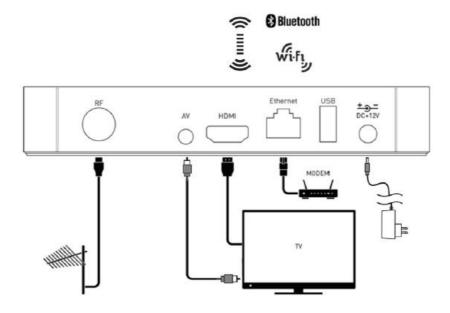
Connect the box to the network either using the LAN connector or via a WiFi connection (802.11 b/g/n/ac; 2.4/5 GHz).
