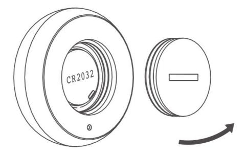
Insert a thin blade or coin into the slot on the battery cover and rotate it anticlockwise to open the battery cover.
