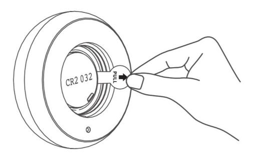
Remove the battery insulation film to power on the product and close the battery cover. 2. Press the reset button for 5S and release, the red LED will flash f or network setting. Use a pin to press the button for 5s.
