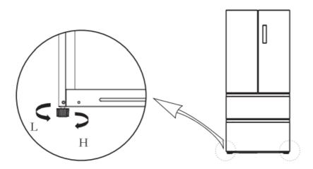
• Schematic diagram of the levelling feet.
