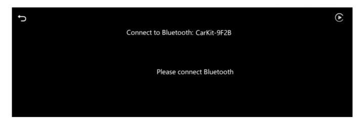
Enter the instrument interface (CarPlay/Auto), open the corresponding icon, and enter the prompt connection interface; Open the Bluetooth on your phone, find the Bluetooth with the name" Carkit -\*\*\*\*, click pairing, and after the automatic connection is successful, the corresponding screen will be displayed
