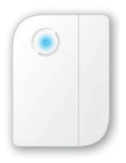
Door/window sensors are used to monitor the open/closed status of doors and windows. Tesla Smart Sensor Door is a wireless ZigBee 3.0 door/window sensor that works with most popular home automation smart controllers and hubs. Use it to control other ZigBee devices (directly) or use it to trigger automation events when doors or windows are opened or closed.
