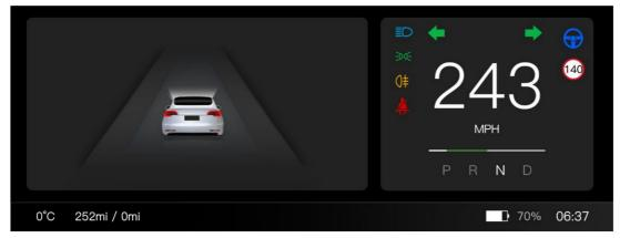
Slide up and down on the left side of the instrument panel to manually adjust the instrument panel speaker volume.
