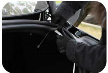
7. As shown in the picture, slowly install the light strip into the rubber strip and follow the direction as shown in the picture (If you are still unclear, you can watch the installation video or contact us)
