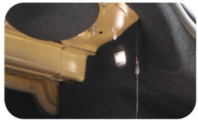
10. Reinstall the lighting and hide the exposed wiring harness in the trim panel.
