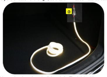
6. Open the rubber strip with your hands and put the light strip in. The bright side cannot be facing inward (The position of the lamp head is also as shown in the picture. At the connection between the upper trim panel and the side trim panel inside the trunk, make sure the power plug harness is long enough to be connected. Just go up)
