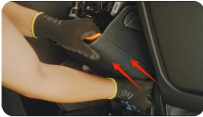
6. Pry open the passenger triangle trim
