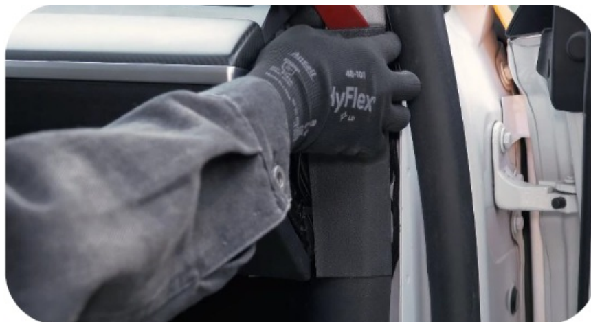
8. Pry open the fixing fastener of the side pedal trim plate, remove the side pedal trim plate and take it out
