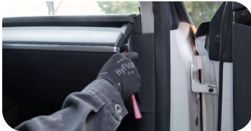
7. Use the warping board to lift the passenger rectangular trim board
