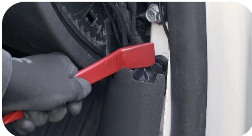
9. Pull down the passenger's side door size
