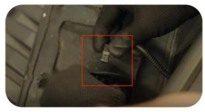
5. Pass the camera harness through the lower grille into the cabin.
