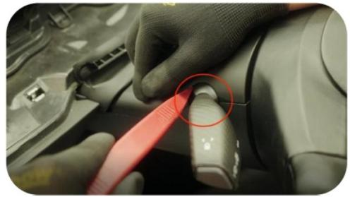
6. Release the clip on the dust-proof leather cover of the steering gear
