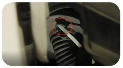
9. Pull out the wiring strap from the passenger side (Tie the wiring harness in the cabin)
