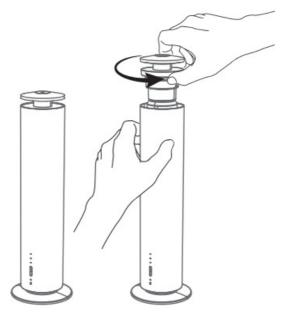
2. Squeeze the atomiser head and rotate the bottle counterclockwise to detach it. After filling the bottle with essential oil, reassemble all components back onto the device and tighten them securely.
