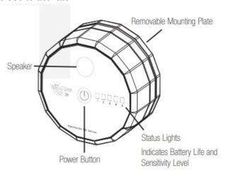
Power On/Off: Press the power button until status lights turn on. Press and hold to turn off.
