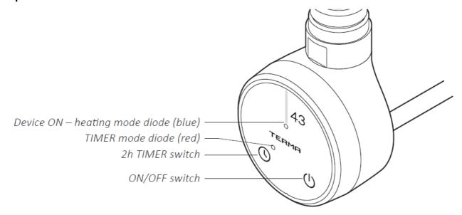
Pressing the key switches the heating element on and the radiator will warm up to an average temperature of approximately 43°C. On the control panel blue LED lights up to indicate the current (ON) status of the heater.
